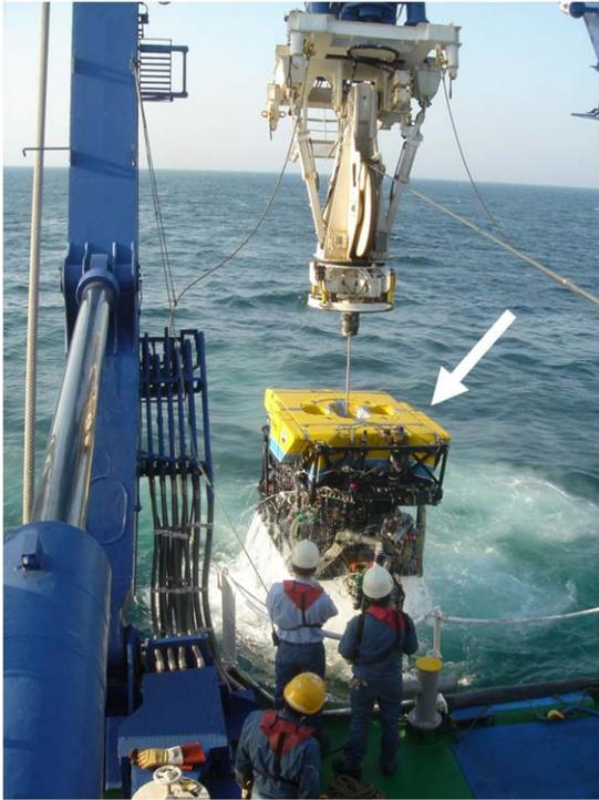
Fig. 2. The remotely operated vehicle, Hyper-Dolphin (arrow).
